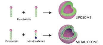
**Scheme 2** Formation of liposomes with phospholipids or metallosomes by mixing metallosurfactants and phospholipids.
