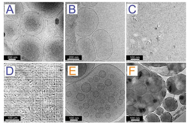
Fig. 2 Images of mixed systems of MTS and SPC. A and B: Cryo-TEM pictures of TCOL6/SPC 1:3 mM/mM vesicles. C: Cryo-TEM image of TCOL6/SPC 3:3 mM/mM bicelles (arrows). D: Optical microscopy picture of TCOL6/SPC 10:3 mM/mM rods. E and F: Cryo-TEM images of PCOL6/SPC vesicles at 6:3 and 10:3 mM/mM, respectively.
