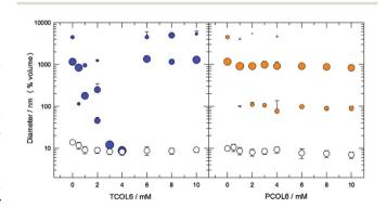
Fig. 1 DLS analysis of the size distribution of TCOL6/SPC aggregates (blue) and PCOL6/SPC aggregates (orange) as a function of the concentration of each MTS (mean  $\pm$  std. dev.;  $n \ge 3$ ). White circles correspond to aggregates obtained after addition of Triton X-100. The SPC concentration was kept constant (3 mM). The area of the circles is proportional to the percentage of aggregates of a given diameter.
