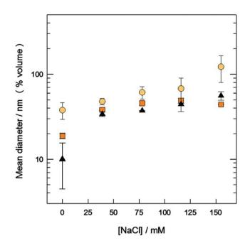
Fig. 5 Mean diameter of PCOL6/SPC 1:3 mM/mM vesicles obtained by microfluidics as a function of the ionic strength of the aqueous medium, using methanol as the solvent, FRR = 3, and TFR = 2 (circles), 10 (squares) and 18 mL min<sup>-1</sup> (triangles). Mean  $\pm$  std. dev.;  $n \ge 2$ .
