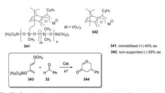
Fig. 82 Reversal of enantioselectivity upon immobilization of an oxovanadium complex in a Diels–Alder reaction.
