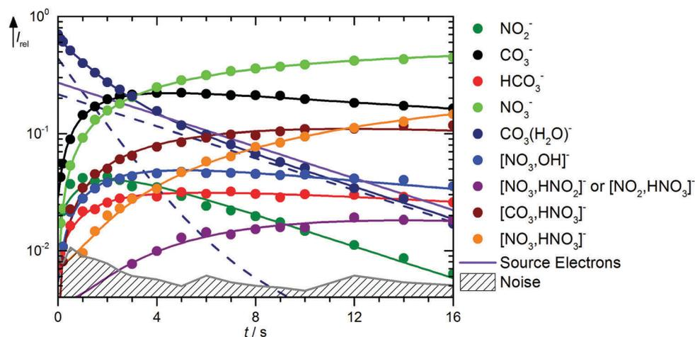
Fig. 3 Kinetics of the reaction of  $\text{CO}_3^{\bullet-}(\text{H}_2\text{O})$  with  $\text{HNO}_3$  and  $\text{H}_2\text{O}$ , with traces of HONO, at a  $\text{HNO}_3$  partial pressure of  $2.1 \times 10^{-8}$  mbar. The lines represent the fit with the rate coefficients from Table S2 (ESI†). Selected mass spectra are shown in Fig. S6 (ESI†).
