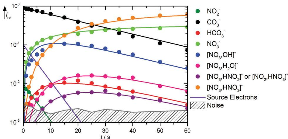
Fig. 2 Kinetics of the reaction of  $\text{CO}_3^{\bullet-}$  with  $\text{HNO}_3$  and  $\text{H}_2\text{O}$ , with traces of HONO, at a  $\text{HNO}_3$  partial pressure of  $1.4 \times 10^{-8}$  mbar. The lines represent the fit with the rate coefficients from Table S1 (ESI<sup>†</sup>). Selected mass spectra are shown in Fig. S5 (ESI<sup>†</sup>).
