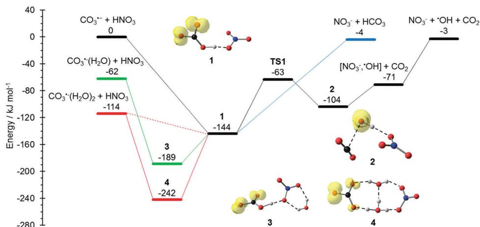
Fig. 1 Reaction potential energy surface (PES) calculated on the M06-2X/6-311++G(d,p) level of theory, with zero-point corrected energies given in kJ mol<sup>-1</sup>. More detailed results on the influence of solvation and additional reaction channels are given in the ESI<sup>†</sup>, Fig. S1–S4.
