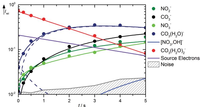
Fig. 4 Kinetics of the reaction of  $\text{CO}_3^*(\text{H}_2\text{O})_2$  with  $\text{HNO}_3$  and  $\text{H}_2\text{O}$ , with traces of HONO, at a  $\text{HNO}_3$  partial pressure of  $8.1 \times 10^{-9}$  mbar. The lines represent the fit with the rate coefficients from Table S3 (ESI†). Selected mass spectra are shown in Fig. S7 (ESI†).
