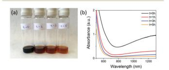
Fig. 1 (a) Picture showing 5 mL aliquots taken from the reaction mixture at (from left to right) t = 0, 1, 3 and 5 hours post-exposure to air. (b) The corresponding loss of absorbance above  $\sim$ 650 nm for the aliquots removed from the reaction mixture.
