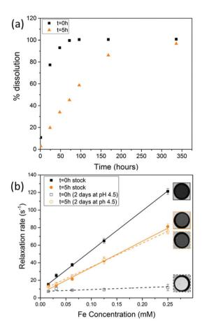
Fig. 3 (a) Dissolution of SPIONs in citrate buffer system at pH 4.5 at 37 °C for 14 days (b)  $T_2^*$  solution relaxivity of SPIONs before and after exposure to citrate buffer for 2 days. MR images correspond to a concentration of 0.25 mM as imaged with a MGE sequence at TE = 15.5 ms.
