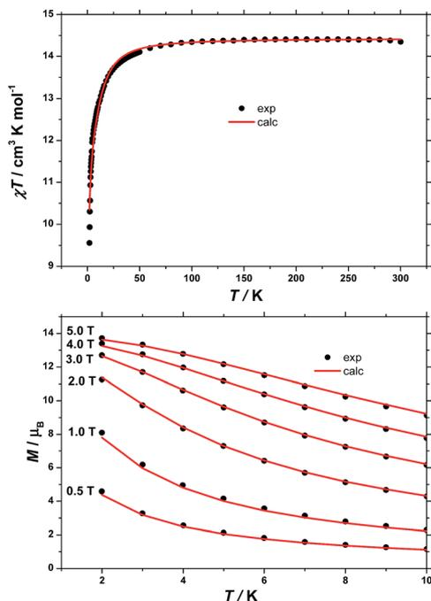
Fig. 5 (Top) Temperature dependence of the  $\chi T$  product of a polycrystalline sample of **1** with  $B = 0.1$  T. (Bottom) VTVB magnetisation data of **1** in the field and temperature ranges 0.5 to 5 T and 2 to 10 K, respectively. Solid lines are the best-fit curves, see text for details.
