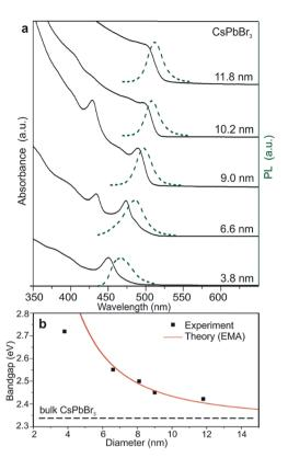
Fig. 10 (a) Quantum-size effects in the absorption and emission spectra of 5-12 nm CsPbBr $_3$  NCs. (b) Experimental *versus* theoretical (effective mass approximation, EMA) size dependence of the band gap energy. Reprinted with permission from ref. 49.
