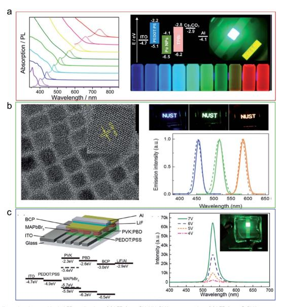
Fig. 12 Low dimensional perovskite in LED applications. (a) LED from  $CH_3NH_3PbX_3$  quantum dots. (b) LED from  $CsPbX_3$  quantum dots. (c) LED from  $CH_3NH_3PbX_3$  nanoplatelets. Reprinted with permission from ref. 17, 90 and 91.
