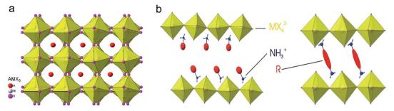
Fig. 1 Structure of 3D and 2D perovskites:  $^{33}$  (a) structure of AMX $_3$  3D perovskite; (b) structure of layered perovskites with (left) monoammonium (RNH $_3^+$ ) or (right) diammonium ( $^+$ H $_3$ N-R-NH $_3^+$ ) organic cations.
