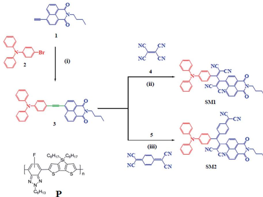
**Scheme 1** Synthesis of triphenylamine-substituted 1,8-naphthalimides **SM1** and **SM2**. Reaction conditions: (i)  $\text{PdCl}_2(\text{PPh}_3)_2$ ,  $\text{CuI}$ ,  $\text{THF} : \text{TEA}$  (1 : 1),  $70^\circ\text{C}$ , 15 h; (ii)  $\text{CH}_2\text{Cl}_2$ ,  $40^\circ\text{C}$ , 20 h. (iii)  $\text{C}_2\text{H}_4\text{Cl}_2$ ,  $100^\circ\text{C}$ , 48 h. The chemical structure of the D–A conjugated polymer is also shown.
