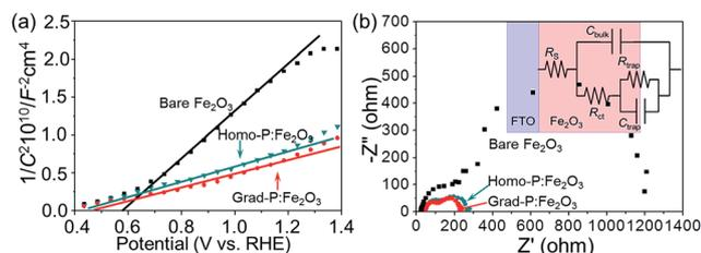
Fig. 6 (a) Mott-Schottky plots and (b) EIS Nyquist plots of bare  $\text{Fe}_2\text{O}_3$ , homo-P: $\text{Fe}_2\text{O}_3$  and grad-P: $\text{Fe}_2\text{O}_3$  photoanodes (inset: equivalent circuit of the photoanode).
