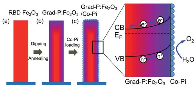
**Scheme 1** Schematic illustration of the synthetic procedure of a grad-P: $\text{Fe}_2\text{O}_3$ /Co-Pi photoanode. (a) Oriented  $\text{Fe}_2\text{O}_3$  nanobundle arrays grown on FTO substrate using RBD; (b) the prepared  $\text{Fe}_2\text{O}_3$  nanobundle arrays were incorporated with gradient P concentrations (the color gradient as an indicator of P content); (c) a thin Co-Pi layer was loaded on grad-P: $\text{Fe}_2\text{O}_3$  photoanode.
