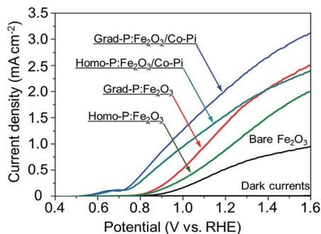
Fig. 4  $I$ - $V$  characteristics of bare  $\text{Fe}_2\text{O}_3$ , homo-P: $\text{Fe}_2\text{O}_3$ , grad-P: $\text{Fe}_2\text{O}_3$ , homo-P: $\text{Fe}_2\text{O}_3/\text{Co-Pi}$  and grad-P: $\text{Fe}_2\text{O}_3/\text{Co-Pi}$  photoanodes measured in 1 M KOH solution under AM 1.5G illumination ( $100 \text{ mW cm}^{-2}$ ). The dark currents are negligible for all samples.
