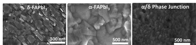
Fig. 4 Top-view scanning electron microscope (SEM) images of the films:  $\delta$ -FAPbI<sub>3</sub>,  $\alpha$ -FAPbI<sub>3</sub> and 1.2 M-FAI with the  $\alpha/\delta$  phase junction.
