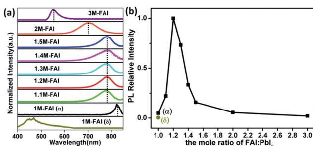
Fig. 2 (a) The normalized PL spectra of the FAPbI<sub>3</sub> films formed with stoichiometrically modified precursor solutions. All the films were excited at 466 nm, except for  $\delta$ -FAPbI<sub>3</sub> at 300 nm. (b) The relative PL intensity of different FAPbI<sub>3</sub> films measured with the integral area of their PL spectra.
