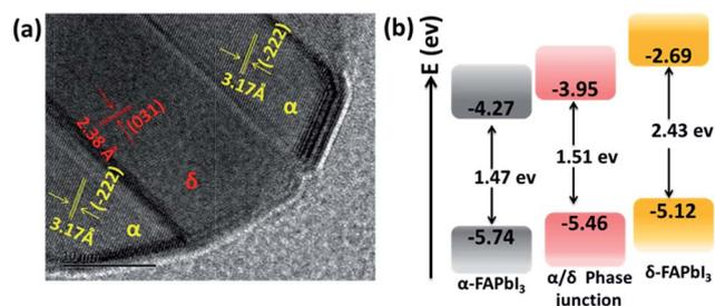
Fig. 3 (a) HRTEM of the 1.2 M-FAI film with the  $\alpha/\delta$  phase junction. (b) Schematic energy level diagrams of the films of pure  $\alpha$ -FAPbI<sub>3</sub>, pure  $\delta$ -FAPbI<sub>3</sub> and the  $\alpha/\delta$  phase junction for the 1.2 M-FAI film.
