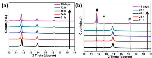
Fig. 6 XRD spectra of the films as a function of time under ambient humid conditions (temperature at 25 °C and relative humidity <50%). (a) The 1.2 M-FAI film with the  $\alpha/\delta$  phase junction, and (b) pure  $\alpha$ -FAPbI<sub>3</sub> annealed at 170 °C. The reflections indicated by \* and # represent the Bragg reflections associated with PbI<sub>2</sub> and  $\delta$ -FAPbI<sub>3</sub>, respectively.
