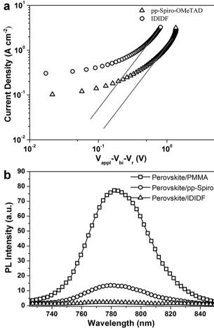
Fig. 4 (a) The space-charge-limited-current (SCLC) of hole-only devices with the configuration of indium tin oxide (ITO)/poly(3,4-ethylenedioxythiophene)-polystyrene sulfonate (PEDOT:PSS)/p,p-spiro-OMeTAD or IDIDF (with Li-bis(trifluoromethanesulfonyl)imide (Li-TFSI) and 4-tert-butylpyridine (tBP) as additives)/Au. (b) PL emission spectra of perovskite/PMMA, perovskite/p,p-spiro-OMeTAD, and perovskite/IDIDF film under excitation at 670 nm.
