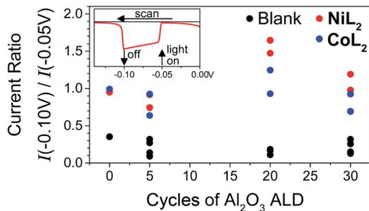
Fig. 5 Ratios of current densities at  $-0.10$  V (light off) to those at  $-0.05$  V (light on) during LSV in duplicate and for NiO|PMI|ALD films with 0–30 cycles of  $Al_2O_3$  ALD (black, "blank") and again after additional 0.5 mM  $NiL_2$  (red) or 0.5 mM  $CoL_2$  (blue). The raw data for the two sets of films are reported in Fig. S13 and S15† (conditions: 0.1 M  $Na_2SO_4$  and 0.1 M  $H_2SO_4$  in 1 : 1  $H_2O$  : MeCN).
