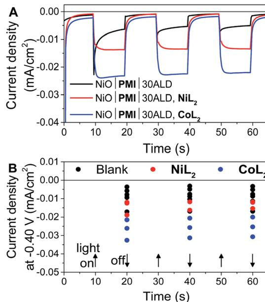
Fig. 6 (A) Current density measurements with three 10 s light on/off cycles with  $-0.40$  V applied bias on a single NiO|PMI|30ALD working electrode without catalyst (black, "blank") and again after additional 0.5 mM  $NiL_2$  (red) or 0.5 mM  $CoL_2$  (blue). (B) Results of the same experiment with 5–30 cycles of  $Al_2O_3$  ALD from Fig. S16.† The number of cycles of ALD is not distinguished for clarity (conditions: 0.1 M  $H_2SO_4$  and 0.1 M  $Na_2SO_4$  in 1 : 1  $H_2O$  : MeCN).
