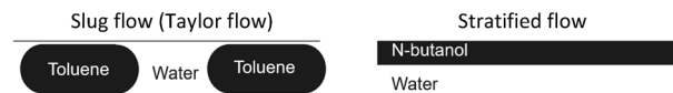
Fig. 1 Two-phase flow patterns observed for the fluid systems toluene–water (left) and n -butanol–water (right) in an empty glass tube. Due to the differences in interfacial tension between the aqueous phase and the organic phase, the two-phase flow of toluene–water is established as slug flow (or Taylor flow), whereas that of n -butanol–water results in stratified flow.
