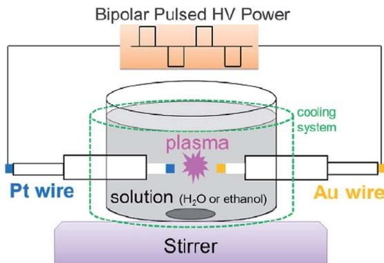
Fig. 14 Image of a synthesis apparatus of a gold/platinum alloy by in-liquid plasma using gold and platinum electrodes. Reproduced from Hua and coworkers.<sup>157</sup> Copyright 2013 by Elsevier.
