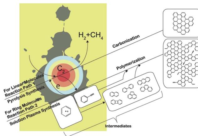
Fig. 17 Reaction routes from hexane, hexadecane, cyclohexane, and benzene. Modified with permission from ref. 164. Copyright 2016 by the Nature Publishing Group.
