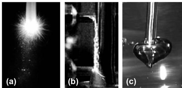
Fig. 19 Method of generating in-liquid plasma for use in water treatment: (a) method of the immersed electrodes in water; (b) method using water flow; (c) method using bubbles. Reproduced from Akiyama *et al.*<sup>220</sup> Copyright 2014 by The Japan Society of Plasma Science and Nuclear Fusion Research.
