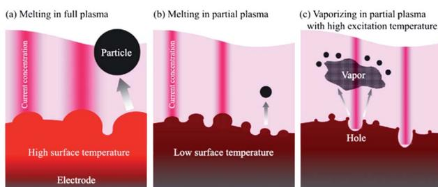
Fig. 13 Images of (a) a wide-area plasma; (b) a partial plasma; and (c) the volatilization of a metal electrode by partial plasma under high temperature conditions. Reproduced from Saito *et al.*<sup>99</sup> Copyright 2014 by the American Institute of Physics.
