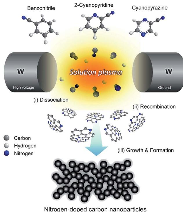
Fig. 16 Schematic illustration of the formation mechanism of nitrogen-doped carbon nanoparticles (NCNPs) *via* a solution plasma process. Modified with permission from ref. 163. Copyright 2016 by Elsevier.
