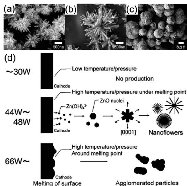
Fig. 15 SEM images of products obtained from in-liquid plasma usage; experimental conditions of  $K_2CO_3$  concentration, and discharge voltage/power are: (a) 1.0 M, 66 V/44 W, (b) 0.5 M, 80 V/48 W, (c) 0.01 M, 200 V/168 W. (d) Schematic processes in the synthesis of ZnO nanoflowers and ZnO aggregates using in-liquid plasma. Modified with permission from ref. 90. Copyright 2011 by Elsevier.
