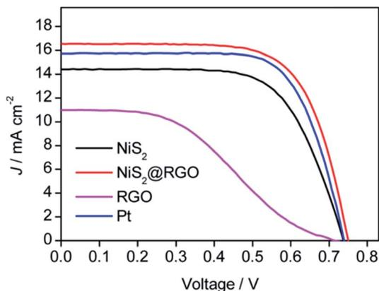
Fig. 15 (a) Photocurrent density–voltage ( $J$ – $V$ ) curves of DSSCs with bare  $\text{NiS}_2$ ,  $\text{NiS}_2$ @RGO nanocomposites, bare RGO, and Pt CEs measured under light illumination of  $100 \text{ mW cm}^{-2}$  (AM 1.5). Reprinted with permission from ref. 210, Z. Li, F. Gong, G. Zhou and Z. S. Wang,  $\text{NiS}_2$ /reduced graphene oxide nanocomposites for efficient dye-sensitized solar cells. *J. Phys. Chem. C*, 2013, **117**, 6561–6566. Copyright© American Chemical Society.
