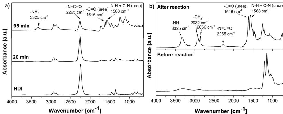
Fig. 2 (A) ATR-FTIR spectra of pure HDI and reaction mixtures after 20 and 95 min of reaction between GO-NH<sub>2</sub> and HDI in *n*-butyl acetate. (B) ATR-FTIR spectra of dried and washed GO-NH<sub>2</sub> before and after reaction with HDI.
