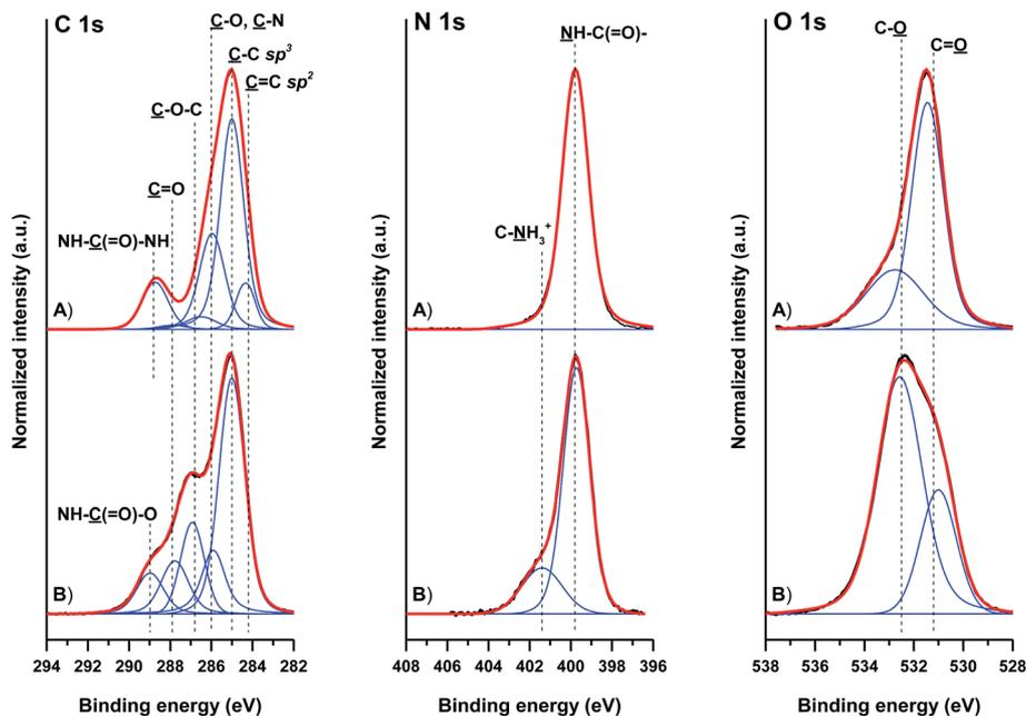
Fig. 4 High-resolution C 1s, N 1s and O 1s XPS spectra of (A) GO-NH<sub>2</sub> and (B) GO reacted with HDI. The measured spectra are presented with black lines, while their corresponding fitted envelopes are presented in red. The individual contributions of different functional groups present in the GO materials are represented with blue lines.
