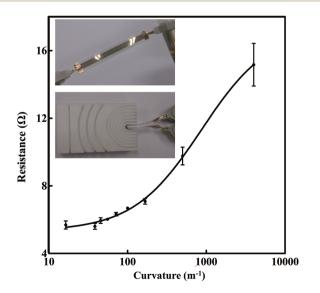
Fig. 8 Resistance of the silver tracks as a function of the bending curvature. All the data for each experimental condition were collected for several-times repetitions. The average values and standard deviation (error bar) were labeled. Photographs of the bending track sample and the measurement details are shown in the insets.
