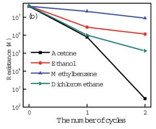
Fig. 4 (a) Comparison of the resistivity of printed silver tracks treated by the MRTP and hot plate heating at  $120\,^{\circ}$ C. (b) Comparison of the resistivity changes of the printed silver tracks treated by Step 1 of MRTP using different organic solvents.
