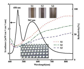
Fig. 5 Irradiance spectra of white light LED and reflectivity spectra of the printed tracks. S1 to S3 represent the reflectivity spectra of the asprepared silver track, the ones treated by Step 1 of MRTP and by Step 2 of MRTP, respectively. The photographs in the insets show the silver tracks of S1 to S3, and the LED light source.
