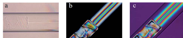
Fig. 6 Glyceryl monooleyl ether (GME) sample in a 0.2 mm diameter quartz capillary under polarized light. (a) Without an analyzer (a polarizer only) (b) and (c) Glyceryl monooleyl ether (GME) sample under polarized light when polarizer and analyzer are perpendicular to each other. Reprinted with permission from ref. 39. Copyright 2016 American Chemical Society.
