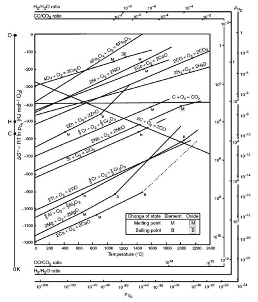
Ellingham-diagram for the formation of oxides based on their standard free energy of formation over temperature.<sup>34</sup>
