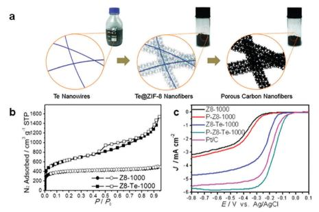
Fig. 6 (a) Illustration of the nanowire-directed templated synthesis of ZIF-8 nanofibers and derived porous doped carbon nanofibers; (b) N<sub>2</sub> sorption isotherms (@77 K) of Z8-Te-1000 and Z8-1000; (c) linear sweep voltammetry (LSV) curves of all catalysts in O2-saturated 0.1 M KOH with a sweep rate of 10 mV s<sup>-1</sup> and electrode rotation speed of 1600 rpm. Reprinted with permission from Zhang et al., 2014. <sup>224</sup> Copyright 2016, American Chemical Society.
