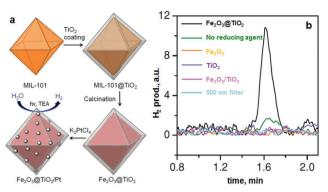
Fig. 4 (a) MOF-templated synthesis of Fe<sub>2</sub>O<sub>3</sub>@TiO<sub>2</sub> by coating MIL-101(Fe) with TiO<sub>2</sub> followed by calcination, and its use for photocatalytic hydrogen production after depositing Pt particles; (b) the H<sub>2</sub> peaks in GC analysis of the headspace using 0.5 mg of different catalyst samples. From de Krafft et al. 2012.  $^{110}$  Copyright  $\odot$  2012 by John Wiley Sons, Inc. Reprinted by permission of John Wiley & Sons, Inc.
