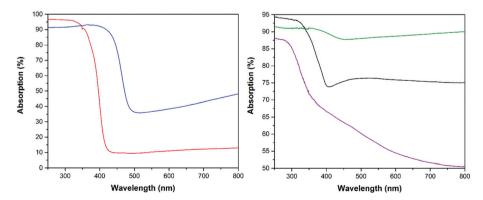
Fig. 3 Absorption spectra of the employed  $WO_3$  (blue) and  $TiO_2$  P25/20 (red) powders (left side) and of the cold sprayed  $Ti/WO_3$  (green) and  $Ti/TiO_2$  (black) photoelectrodes (right side). The purple curve on the right side shows the absorption spectra of the employed blank Ti substrate.
