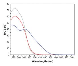
Fig. 14 IPCE spectra for methanol oxidation employing cold sprayed  $WO_3$  (blue) and  $TiO_2$  (red) on titanium metal photoanodes. The IPCE curve of screen printed  $TiO_2$  on FTO photoelectrode is also given (light grey) for comparison. Measurements for methanol oxidation were conducted in an aqueous solution of 0.5 M  $H_2SO_4$  with addition of 10 vol% of methanol (~2 mol  $L^{-1}$ ) at a bias of 1 V vs. NHE.
