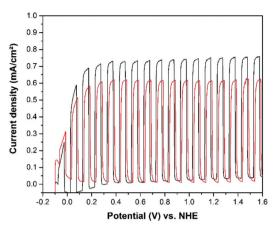
Fig. 7 Chopped light current–potential curves of cold sprayed  $\text{TiO}_2$  on titanium metal (red) and screen printed  $\text{TiO}_2$  on FTO (black) photo-anodes in 0.5 M  $\text{H}_2\text{SO}_4$  with addition of 10 vol% of methanol (~2 mol L<sup>-1</sup>). Measured with a scan rate of 20 mV s<sup>-1</sup>. Current densities were measured upon irradiation with AM 1.5-global light (300 W Xe lamp).
