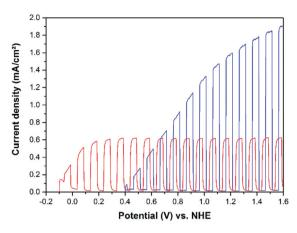
Fig. 12 Chopped light current–potential curves of cold sprayed WO<sub>3</sub> (blue) and TiO<sub>2</sub> (red) on titanium metal photoanodes in 0.5 M  $\rm H_2SO_4$  with addition of 10 vol% of methanol (~2 mol L<sup>-1</sup>). Measured with a scan rate of 20 mV s<sup>-1</sup>. Current densities were measured upon irradiation with AM 1.5-global light (300 W Xe lamp).
