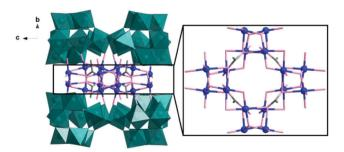
Fig. 1 Representation of the polyanion cluster of 1 (left) and the {Cu<sub>16</sub>} core in the cluster (right). The  $\{W_{11}\}$  building units are shown as teal polyhedra, Cu as blue sphere, O and C as rose and grey sticks
