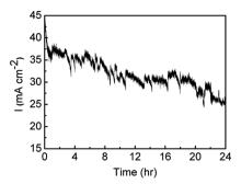
Fig. 9 Stability measurements of Au/Co(OH)<sub>2</sub> held at 1.67 V for 24 h in 1 M NaOH
