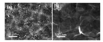
Fig. 2 (a and b) SEM images of Co(OH)<sub>2</sub> electrodeposited on to a Au electrode at a potential of -0.95 V for 60 s in a solution of 10 mM Co(NO<sub>3</sub>)<sub>2</sub>·6H<sub>2</sub>O.
