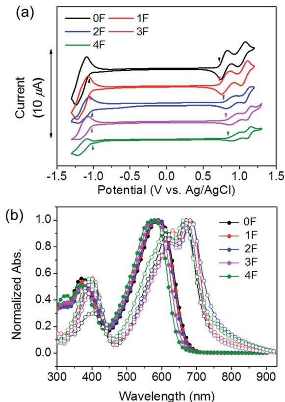
Fig. 1 (a) Cyclic voltammograms of 0–4F dichloromethane solutions containing  $0.1 \text{ mol L}^{-1} \text{ Bu}_4\text{NPF}_6$  and a scan rate of  $50 \text{ mV s}^{-1}$ . (b) UV-vis absorption spectra of 0–4F chloroform solutions (filled circles) and films (open circles).
