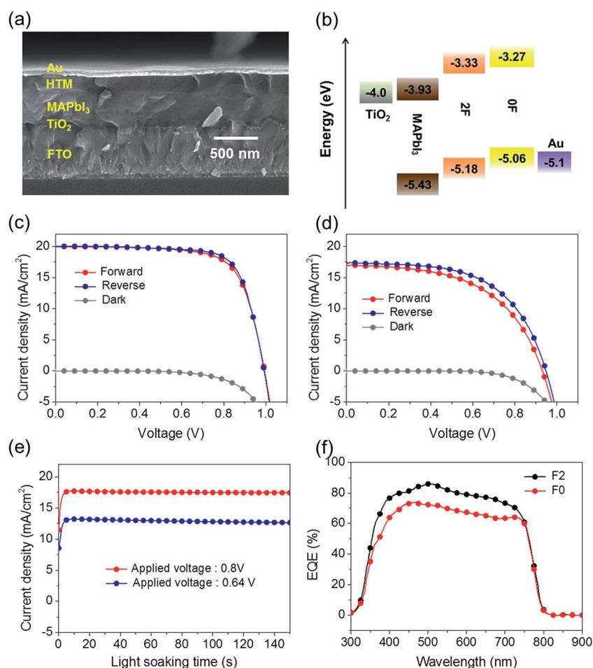
Fig. 7 (a) The SEM cross-section image and (b) energy diagram of the perovskite solar cell device. The current density–voltage (*J*–*V*) characteristics based on the solar cells with (c) **2F** and (d) **0F**. (e) current density (*J*) variation of the **0F** and **2F** based PSCs with a light soaking (1 Sun) time under the applied bias voltage ( $V_{opt}$ ) at maximum power point ( $P_{max}$ ) and (f) EQE spectra of the **0F** and **2F** based PSCs.
