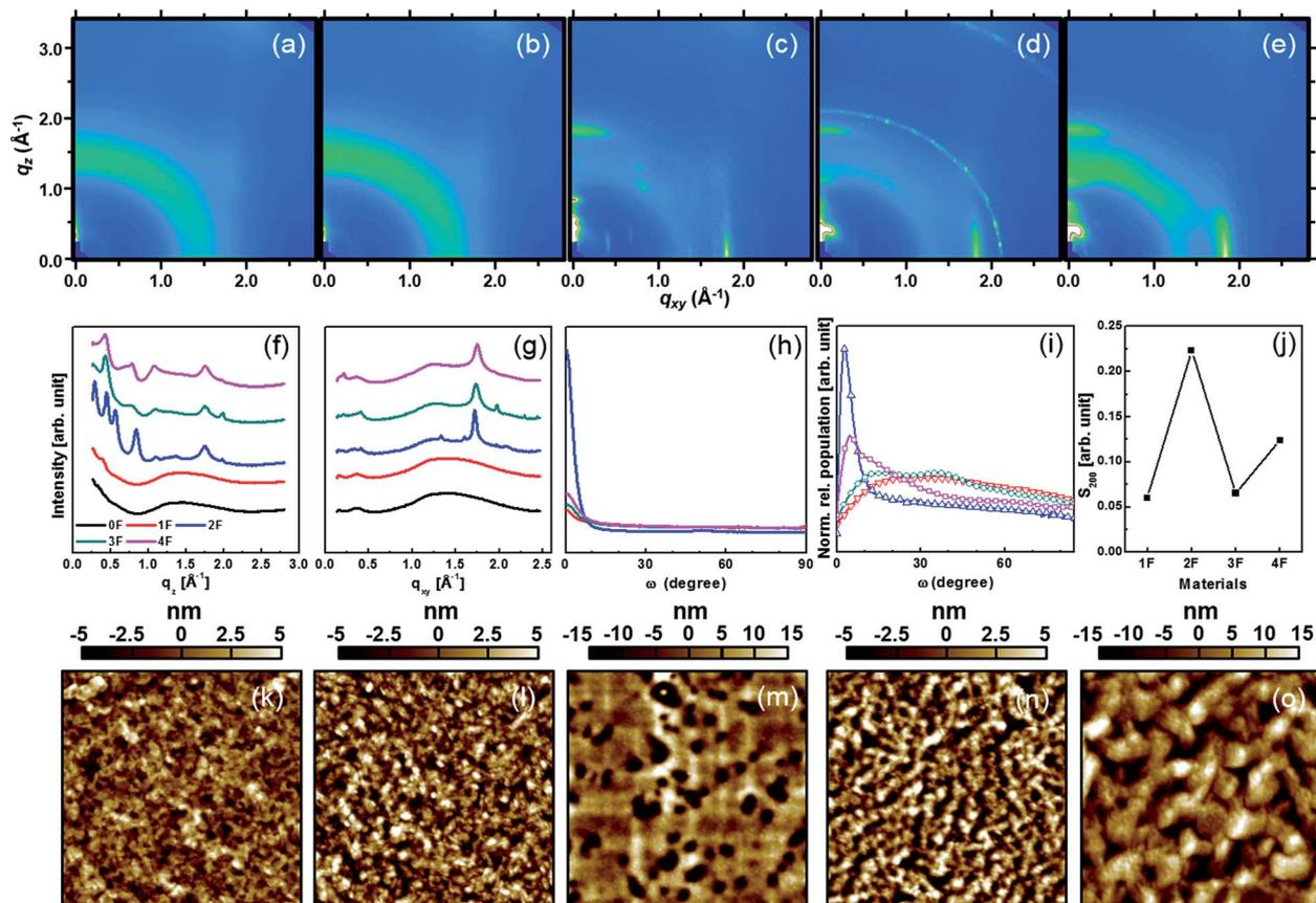
Fig. 4 2D-GIXD patterns of (a) 0F, (b) 1F, (c) 2F, (d) 3F, and (e) 4F films, GIXD patterns in (f) out-of-plane and (g) in-plane directions, (h) the pole figures, (i) the pole figures multiplied by a factor of  $\sin \omega$ , and (j) the Herman's orientation factors as a function of the number of fluorine substitutions. AFM topography images of films consisting of (k) 0F, (l) 1F, (m) 2F, (n) 3F, and (o) 4F.
