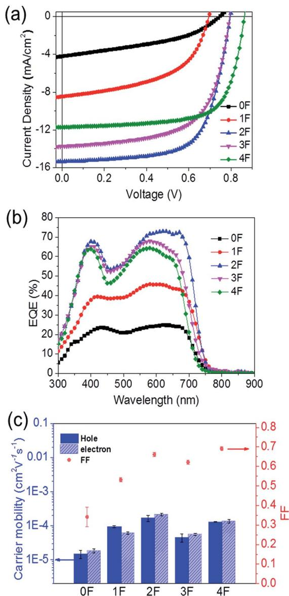
Fig. 5 (a) The current density–voltage ( $J$ – $V$ ) characteristics and (b) external quantum efficiency (EQE) curves based on the 0F–4F/PC<sub>71</sub>BM devices. (c) Comparisons of SCLC hole and electron mobilities of the 0F–4F:PC<sub>71</sub>BM films, and the fill factor values of 0F–4F.
