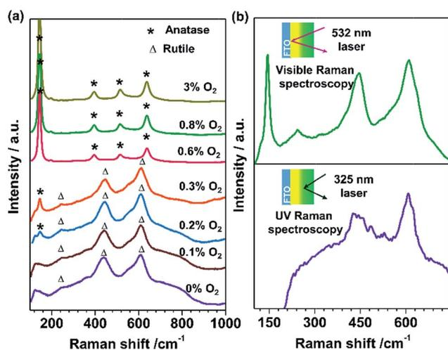
Fig. 2 (a) Visible Raman spectra of the  $\text{TiO}_2$  films fabricated at different  $\text{O}_2$  partial pressures. (b) Visible and UV Raman spectra of the  $\text{TiO}_2\text{-AR}$  electrode, which consists of an internal anatase phase  $\text{TiO}_2$  layer and external rutile phase  $\text{TiO}_2$  layer.
