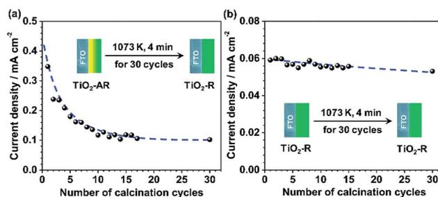
Fig. 6 Dependence of the current density values of  $\text{TiO}_2\text{-AR}$  electrode (a) and  $\text{TiO}_2\text{-R}$  electrode (b) on the number of calcination cycles. After calcination treatment at 1073 K for 120 min (4 minutes per cycle and 30 cycles), the  $\text{TiO}_2\text{-AR}$  was converted to pure rutile phase.
