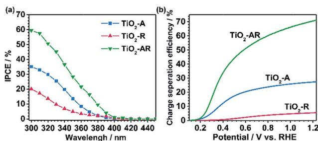
Fig. 5 (a) The incident photon-to-electron conversion efficiency (IPCE) values of  $\text{TiO}_2\text{-A}$  (blue),  $\text{TiO}_2\text{-R}$  (red) and  $\text{TiO}_2\text{-AR}$  (green). (b) The carrier separation efficiencies of  $\text{TiO}_2\text{-A}$  (blue),  $\text{TiO}_2\text{-R}$  (red) and  $\text{TiO}_2\text{-AR}$  (green).
