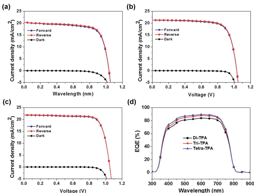
Fig. 5 Photovoltaic properties of planar MAPbI<sub>3</sub> hybrid solar cells with (a) di-TPA, (b) tri-TPA, and (c) tetra-TPA and (d) EQE spectra.
