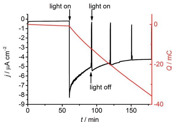
Fig. 5 CPPE of a NiO|RuP3–Zr<sup>4+</sup>–NiP photoelectrode (1 cm<sup>2</sup>) at  $E_{\text{appl}} = 0.3$  V vs. RHE in Na<sub>2</sub>SO<sub>4</sub> (0.5 M, pH 3) at room temperature. Electrolysis was performed in a 2-compartment PEC cell with the working and counter compartment separated by a Nafion membrane. The working electrode was held in the dark for 1 h, followed by irradiation for 2 h using a solar light simulator (100 mW cm<sup>-2</sup>, AM1.5G filter,  $\lambda > 400$  nm).
