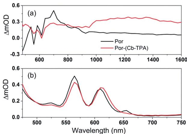
Fig. 5 (a) Transient absorption spectra of TiO<sub>2</sub>-Por and TiO<sub>2</sub>-Por-(Cb-TPA) in the presence of the inert electrolyte I<sub>0</sub> at 10 μs time delay following laser excitation (532 nm, 24–26 μJ cm<sup>-2</sup> per pulse) and (b) absorbance of TiO<sub>2</sub>-Por and TiO<sub>2</sub>-Por-(Cb-TPA).
