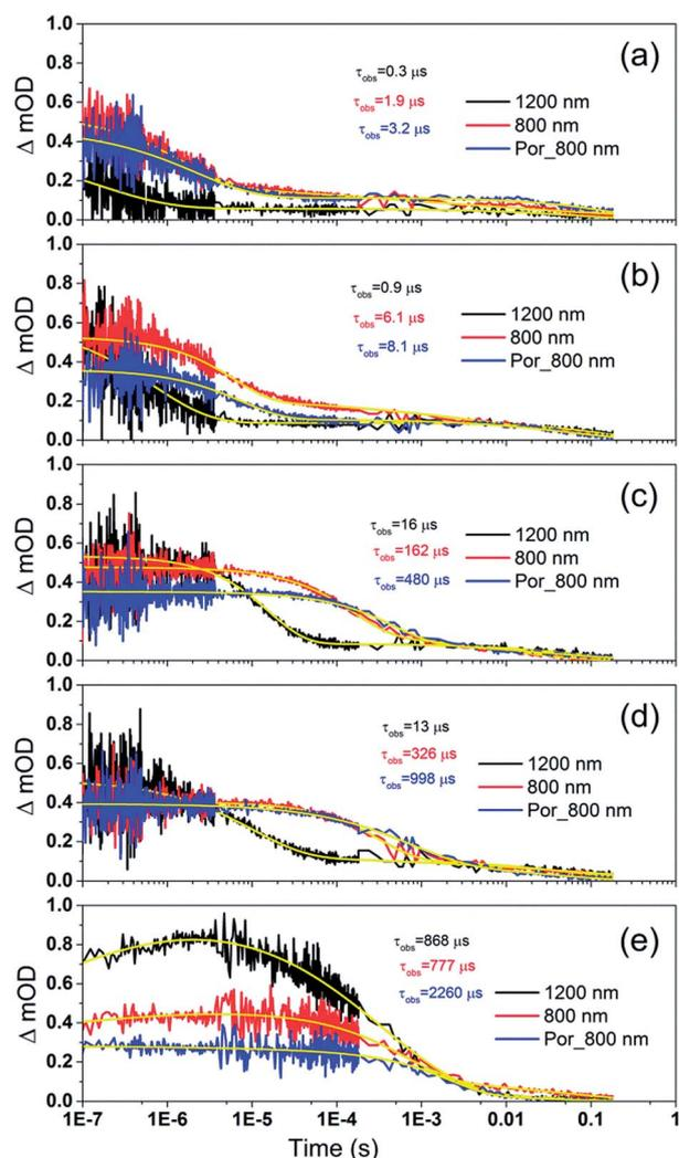
Fig. 7 Transient absorption decay and fitted curves of  $\text{TiO}_2\text{-Por-(Cb-TPA)}$  probed at 1200 nm (black) and 800 nm (red) and  $\text{TiO}_2\text{-Por}$  probed at 800 nm (blue) with five  $\text{I}^-/\text{I}_3^-$  electrolytes after pulsed 532 nm laser irradiation. (a)  $\text{I}_1$ , (b)  $\text{I}_{0.1}$ , (c)  $\text{I}_{0.01}$ , (d)  $\text{I}_{0.001}$  and (e)  $\text{I}_{0.0001}$  (532 nm, 45–50  $\mu\text{J cm}^{-2}$  per pulse; repetition rate 1 Hz).
