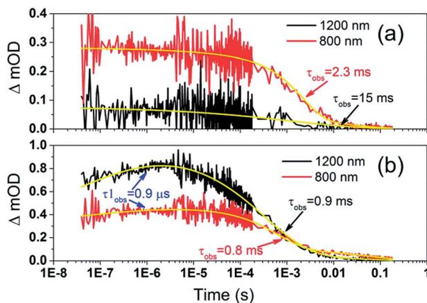
Fig. 6 Transient absorption decays and fitted functions of (a) TiO<sub>2</sub>-Por and (b) TiO<sub>2</sub>-Por-(Cb-TPA) with the inert electrolyte I<sub>0</sub> (532 nm, 45–50 μJ cm<sup>-2</sup> per pulse; repetition rate 1 Hz).
