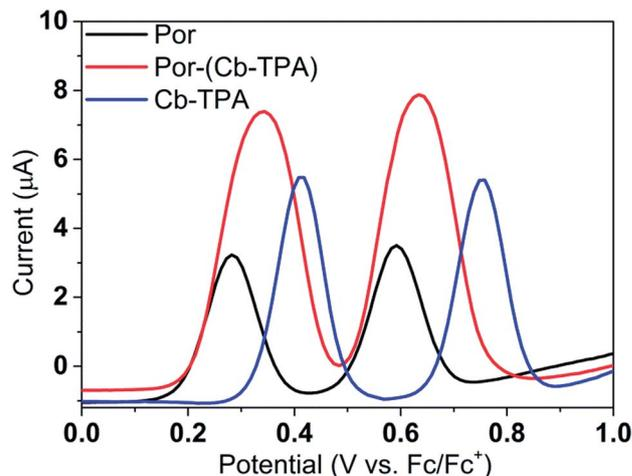
Fig. 3 (a) Differential pulse voltammetry of the compounds measured in dichloromethane solutions.
