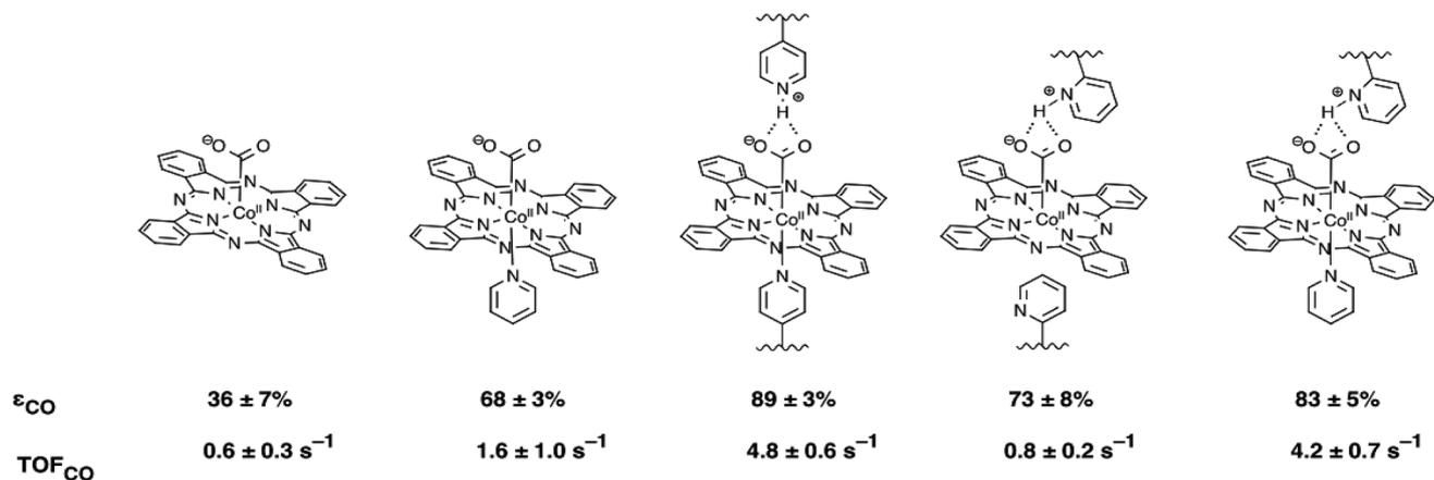
Fig. 7 Proposed activated CO<sub>2</sub> complexes and secondary coordination sphere interaction for each catalyst film studied. Also shown are the faradaic efficiencies and turnover frequencies for each catalyst system determined from CPE measurements.
