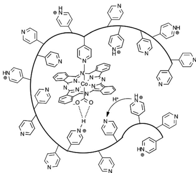
**Fig. 5** An illustration of CoPc immobilized in P4VP. Three properties of the polymer membrane which are suggested to be important to the activity and selectivity of CoPc-PVP are illustrated. Pyridine residues that can coordinate to CoPc, the ability for uncoordinated pyridine residues to act as proton relays, and the hydrogen bonding interactions that may occur between protonated pyridines and activated CO<sub>2</sub>.
