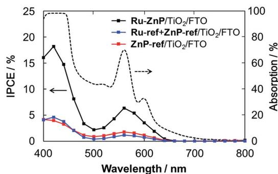
Fig. 5 Photocurrent action spectra of the Ru-ZnP/TiO<sub>2</sub>/FTO (black), Ru-ref + ZnP-ref/TiO<sub>2</sub>/FTO (blue) and ZnP-ref/TiO<sub>2</sub>/FTO electrodes (red) with a TiO<sub>2</sub> thickness of 6 μm. Dashed line depicts the light-harvesting efficiency of the Ru-ZnP/TiO<sub>2</sub>/FTO electrode. Conditions: external bias: -0.2 vs. NHE, electrolyte: PB (0.1 M, initial pH 7.3); and scan rate: 2 nm s<sup>-1</sup> from 400 nm to 800 nm.
