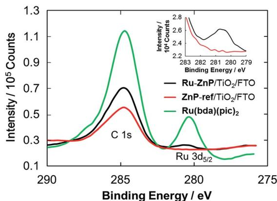
Fig. 3 C 1s and Ru 3d<sub>5/2</sub> XPS spectra of **Ru-ZnP**/TiO<sub>2</sub>/FTO (black), **ZnP-ref**/TiO<sub>2</sub>/FTO (red) and Ru(bda)(pic)<sub>2</sub> (green). Inset is the magnified spectra of **Ru-ZnP**/TiO<sub>2</sub>/FTO (black) and **ZnP-ref**/TiO<sub>2</sub>/FTO (red) for the Ru 3d<sub>5/2</sub> region.
