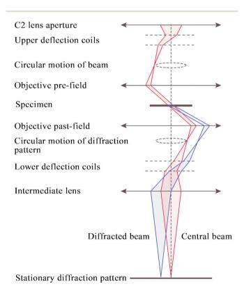
Fig. 6 Schematic ray diagram for precession electron diffraction (PED), illustrating the rocking/de-rocking action of the beam before and after the specimen.<sup>65</sup>
