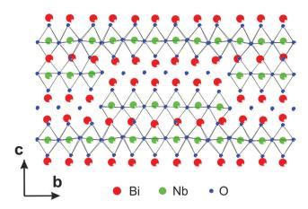
Fig. 13 Part of the structure of Bi<sub>5</sub>Nb<sub>3</sub>O<sub>15</sub> showing both the continuous and discontinuous perovskite blocks and [Bi2O2] slabs. Reproduced with permission from ref. 115. Copyright 2013 American Chemical Society.
