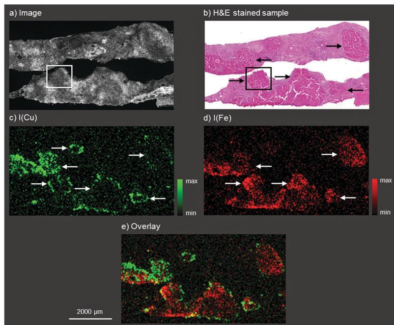
**Fig. 1** Autofluorescence microscopic image of the WD liver sample investigated by bench-top  $\mu$ XRF (a), bright field microscopy image of a H&E stained parallel section of the WD liver sample (b), distribution maps of copper (c) and iron (d), and overlay of the copper and iron distribution (e). The area marked with the white box in a and the black box in b corresponds to the area of the parallel section analyzed later by means of SR- $\mu$ XRF (Fig. 2).
