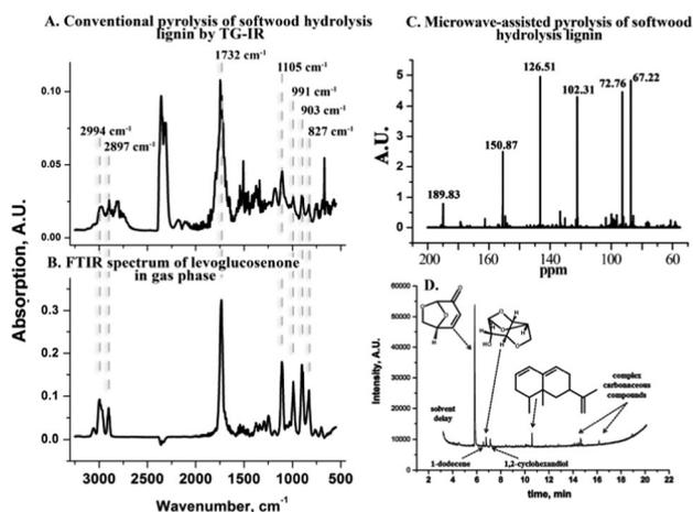
Fig. 1 (A) FT-IR spectrum of the volatiles from conventional pyrolysis of crude waste softwood hydrolysis lignin (CSHL) at 310 °C. (B) Gas phase FT-IR spectrum of LGE. (C) <sup>13</sup>C NMR spectrum of the liquid extract from MW-assisted pyrolysis of CSHL with labelled LGE peaks. (D) GC-MS of the liquid extract from the MW-assisted pyrolysis of CSHL.
