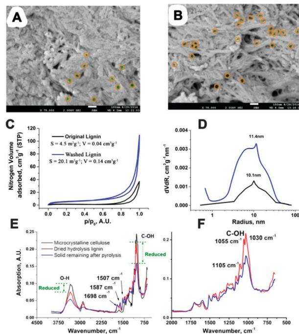
Fig. 4 (A) SEM of original CSHL x75000 with yellow encircled mesopores (B) SEM of washed CSHL x75000 with indicated mesopores (C)  $\text{N}_2$  adsorption isotherms of washed/original CSHL. (D) Pore distribution derived from  $\text{N}_2$  adsorption data for washed/original CSHL. (E and F) FT-IR of original CSHL (dried), the solid remaining after MW heating of CSHL and subsequent extraction of LGE (dried solid) and microcrystalline cellulose.
