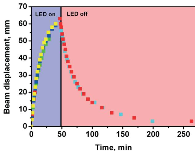
Fig. 4 Illustration of the reproducibility of results over multiple irradiation/heating (photoisomerisation/reverse thermoisomerisation) cycles; crystal #2,  $T = 363$  K. The displacement of the reflected beam on irradiation of the crystal by light from the LED for 50 minutes is shown (rising curve), and that resulting from a subsequent reverse thermoisomerisation in the dark (downward curve).
