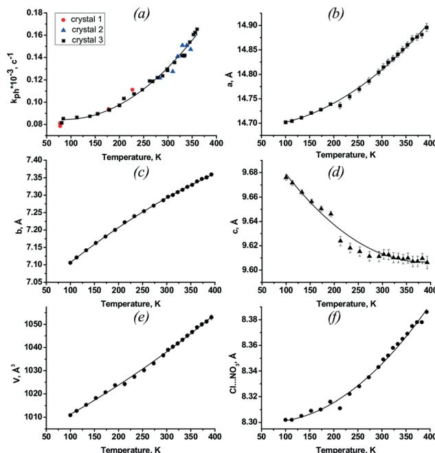
Fig. 6 The temperature dependences of: a) the rate constant of photoisomerisation  $k_{\text{ph}}$ ; b–e) unit cell parameters  $a$ ,  $b$ ,  $c$  and volume  $V$ ; f) the distance between the anions Cl and  $\text{NO}_3$ , surrounding a nitro-ligand  $\text{NO}_2$  (see Fig. 1).
