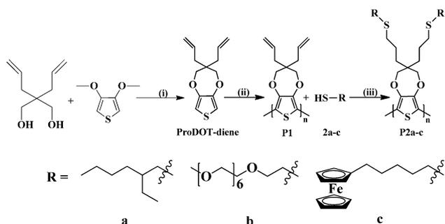
Scheme 1 Synthesis of ProDOT-diene (**1**), electrochemical polymerization of (**1**) to form poly(ProDOT-diene) (**P1**) and “click” reaction of **P1** with various thiols **2a–c** to form **P2a–c**. (i) *p*TSA in toluene at 100  $^{\circ}\text{C}$  for 2 days (ii) ACN–TBAP; (iii) 0.1% DMAP, UV 365 nm, room temperature.
