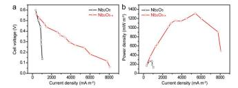
Fig. 5 Comparisons of (a) polarization curves and (b) power outputs for  ${\rm Nb_2O_5}$  and  ${\rm Nb_2O_{5-x}}$  anodes.
