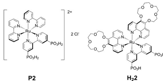
Fig. 1 Molecular structures of **P2**, isolated as its chloride salt, and **2**, obtained in its doubly deprotonated, neutral form **H<sub>2</sub>2**.
