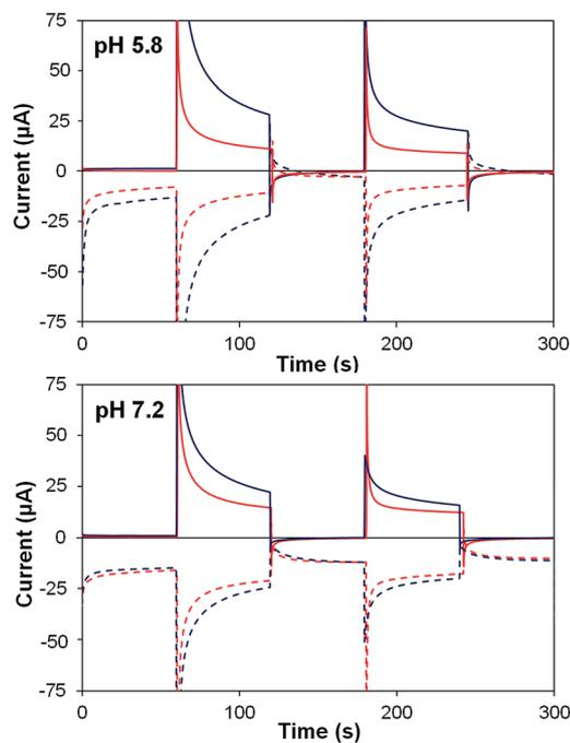
Fig. 7 Photoelectrochemical generator–collector measurements (chronoamperometry) of  $\text{TiO}_2\text{-2}$  (red) and  $\text{TiO}_2\text{-2Na}_2\text{-1}$  (dark blue) at pH 5.8 and pH 7.2. Solid lines are the photoanode current; dashed lines, collector current; collector efficiency *ca.* 60%. Applied bias 0 mV vs. Ag/AgCl, illuminated with a 455 nm LED ( $33 \text{ mW cm}^{-2}$ ). Photocurrent densities are reported in Table 4.
