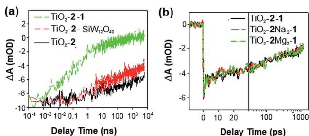
Fig. 5 (a) Ground state bleach recovery kinetics of  $\text{TiO}_2\text{-2}$  (black),  $\text{TiO}_2\text{-2-SiW}_{12}\text{O}_{40}$  (red) and  $\text{TiO}_2\text{-2-1}$ . (b) Ground state bleach recovery kinetics of  $\text{TiO}_2\text{-2-1}$  (black),  $\text{TiO}_2\text{-2-Na}_2\text{-1}$  (red) and  $\text{TiO}_2\text{-2-Mg}_2\text{-1}$  (green).
