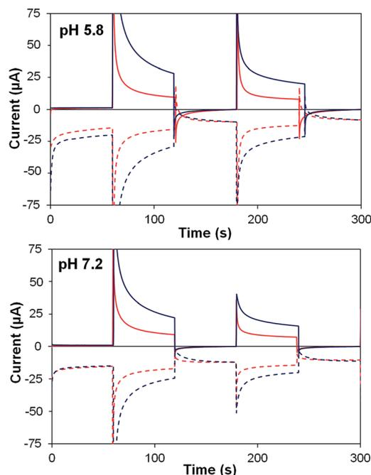
Fig. 8 Photoelectrochemical generator–collector measurements (chronoamperometry) of  $\text{TiO}_2\text{-P2-1}$  (red) and  $\text{TiO}_2\text{-2Na}_2\text{-1}$  (dark blue) at pH 5.8 and pH 7.2. Solid lines, photoanode current; dashed lines, collector current; collector efficiency *ca.* 60%. Applied bias 0 mV vs. Ag/AgCl, illuminated with a 455 nm LED ( $33 \text{ mW cm}^{-2}$ ). Photocurrent densities are reported in Table 5.
