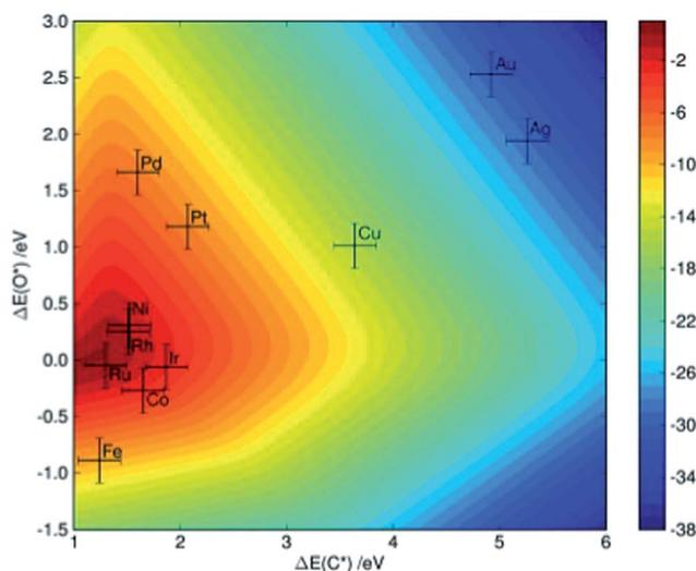
Fig. 4 Two-dimensional volcano-curve of the turnover frequency ( $\log_{10}$ , at  $773 \text{ K}$ ,  $1 \text{ bar}$ ) as a function of C and O binding energy. Reprinted with permission from ref. 7. Copyright 2008 Elsevier.
