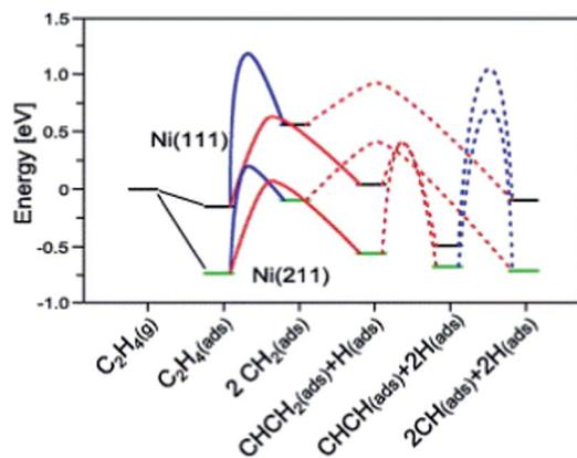
Fig. 7 Potential energy diagram for C–C bond breaking (blue line) and C–H bond breaking (red line) on Ni(111) and Ni(211). The transition state energy for C–H bond breaking of  $\text{CH}_2$  is for one  $\text{CH}_2$ . Reprinted with permission from ref. 90. Copyright 2006 Elsevier.
