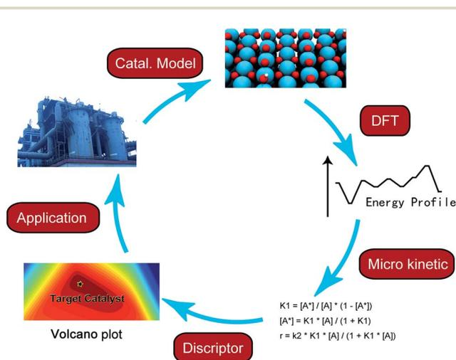
Fig. 1 Scheme of computer aided catalyst design.
