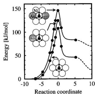
Fig. 10 The calculated energy along the reaction path for CH<sub>4</sub> dissociating over a Ni atom in the Au/Ni(111) surface. The rightmost data points (dashed curves) refer to infinite separation of the dissociated H and CH<sub>3</sub> group on the surface. The dissociation geometry for the three chemical compositions is indicated by the insets, with gold atoms gray-shaded. Reprinted with permission from ref. 37. Copyright 1996 American Institute of Physics Publishing LLC.
