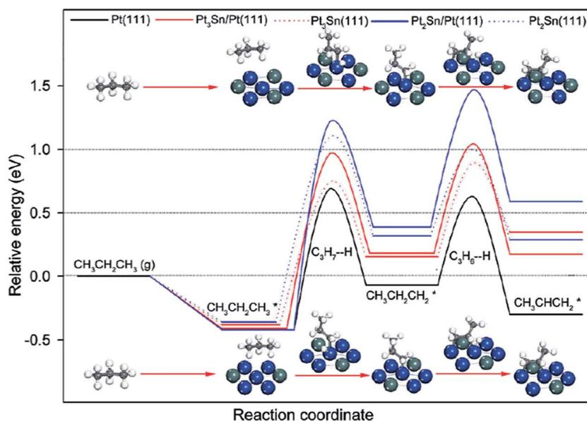
Fig. 12 Energy profiles for propane dehydrogenation to propylene on Pt and PtSn surfaces. Reprinted with permission from ref. 104. Copyright 2012 American Chemical Society.
