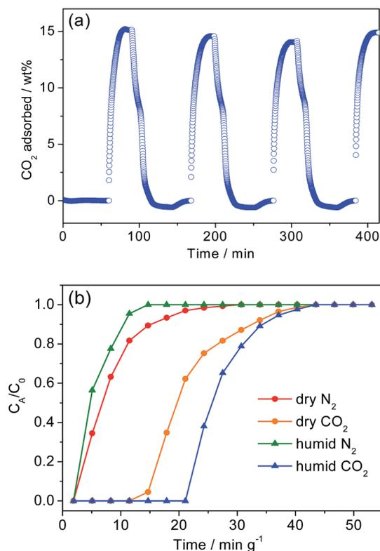
Fig. 5 (a) CO<sub>2</sub> adsorption–desorption cycling curve for **1-dmen** in humid conditions. (b) Breakthrough curves for **1-dmen** under dry (N<sub>2</sub>, red circle; CO<sub>2</sub>, orange circle) and humid conditions (N<sub>2</sub>, green triangle; CO<sub>2</sub>, blue triangle).
