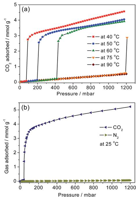
Fig. 2 (a) Adsorption isotherms of CO<sub>2</sub> for **1-dmen** at the indicated temperatures. The solid lines are eye-guides. (b) CO<sub>2</sub> and N<sub>2</sub> isotherms at 25 °C.
