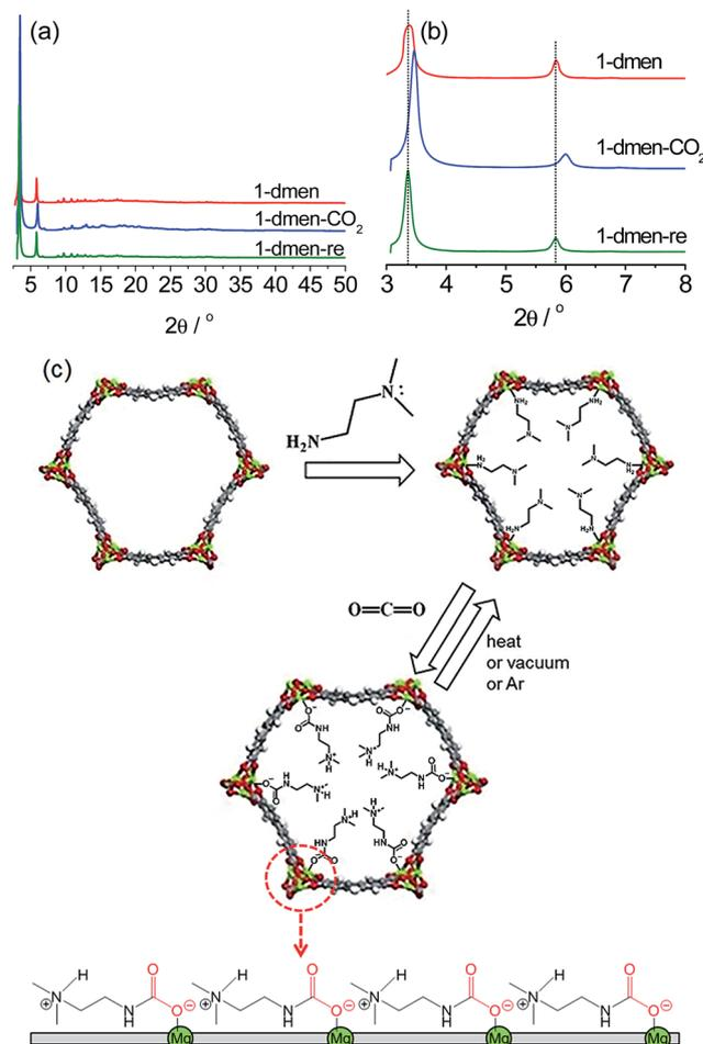
Fig. 1 (a) Synchrotron PXRD profiles of **1-dmen**, **1-dmen-CO<sub>2</sub>**, and **1-dmen-re**. (b) Enlargement of the low-angle region of the PXRD data. (c) Framework structure of **1** with open metal sites, grafting modes of dmen onto the open metal sites, and subsequent CO<sub>2</sub> adsorption. The schematic diagram (bottom) indicates the arrangement of ammonium carbamates running along the *c*-axis.
