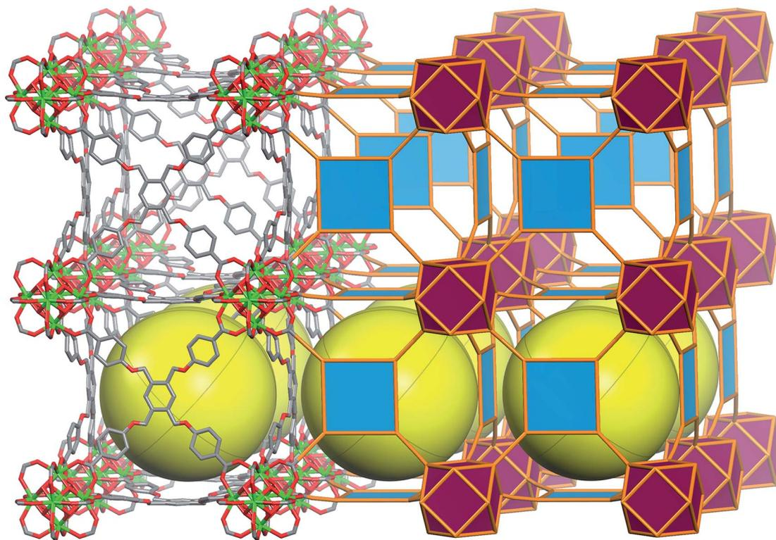
Fig. 4 Molecular and vertex figure representation of **ftw**-MOF-1, yellow spheres denote the open space within each cage; (top left) TetPOMB ligand coordinated to four 12-connected hexanuclear clusters and (bottom right) vertex figure representation.<sup>11</sup>
