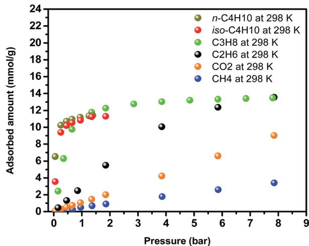
Fig. 7 Single-gas adsorption isotherms for CO<sub>2</sub>, CH<sub>4</sub>, C<sub>2</sub>H<sub>6</sub>, C<sub>3</sub>H<sub>8</sub>, *n*-C<sub>4</sub>H<sub>10</sub> and *iso*-C<sub>4</sub>H<sub>10</sub> on Y-ftw-MOF-2.
