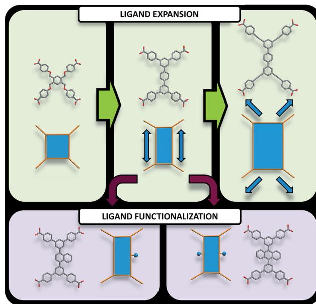
Fig. 3 Pathways to modify quadrangular ligands for the synthesis of **ftw**-MOFs, including examples of ligands and their vertex figures. (Top) Modification of the organic quadrangular MBB through ligand expansion. (Bottom) Modification of the quadrangular organic MBB through ligand functionalization.
