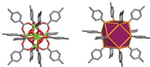
Fig. 1 Left, the 12-connected rare earth hexanuclear cluster,  $[\text{RE}_6(\mu_3\text{-OH})_8(\text{O}_2\text{C-})_{12}]$ .<sup>11</sup> Right, illustration of the MBB coordination geometry: note the positions of the carbon atom of the carboxylates match the vertices of the cuboctahedron.
