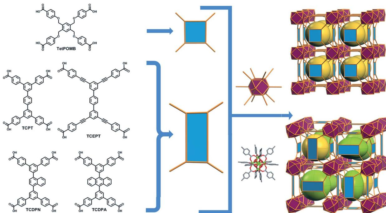
Fig. 2 Schematic showing the assembly of **ftw**-MOFs by combining 4-connected ligands (TetPOMB, TCPT, TCEPT, TCDPN, and TCDPA) with 12-connected rare earth hexanuclear MBBs (with a square or rectangle combined with a cuboctahedron vertex figure respectively), resulting in the **ftw** topology shown here as the augmented **ftw** net.
