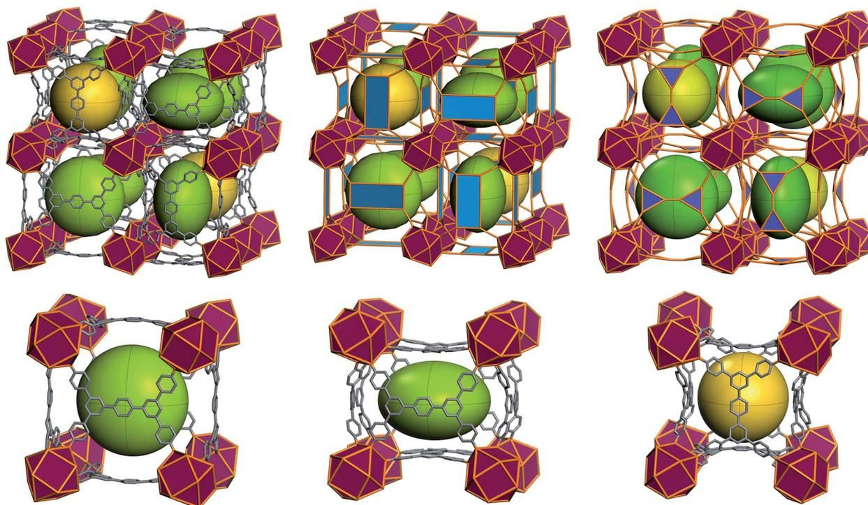
Fig. 6 (Top) Representation of the **ftw**-MOF-2 framework: green ellipsoids represent the larger asymmetrical cage; yellow spheres represent the smaller symmetrical cages. Purple polyhedra represent the rare earth hexanuclear MBB; blue polygons represent the 4-connected quadrangular organic MBB. (Bottom left and center) Diagram of the asymmetrical cage along two axes; (bottom right) diagram of the symmetrical cage.
