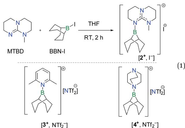
To test this hypothesis,  $[2^+, I^-]$  was synthesized in 81% yield by nucleophilic displacement of the iodine atom in BBN-I by MTBD in THF (eqn (1)). The  $^{11}\text{B}\{^1\text{H}\}$  NMR spectrum of  $2^+$  displays a resonance at +57.2 ppm, consistent with the structure of an electrophilic tricoordinate boron center. This  $^{11}\text{B}$  chemical
