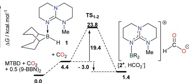
Scheme 1 Computed pathway (M05-2X/6-31+G\*) in THF for the rate-determining step in the MTBD-catalyzed hydroboration of CO<sub>2</sub> to formate.
