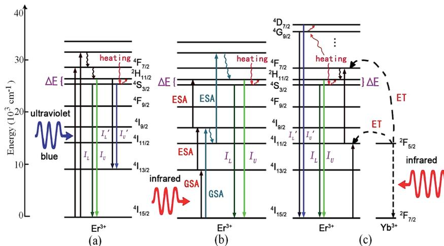
Fig. 3 The mechanism of optical thermal sensing through (a)  $\text{Er}^{3+}$  down-conversion under ultraviolet (blue) excitation, (b)  $\text{Er}^{3+}$  up-conversion under infrared excitation, and (c)  $\text{Yb}^{3+}$ – $\text{Er}^{3+}$  energy transfer under infrared excitation.
