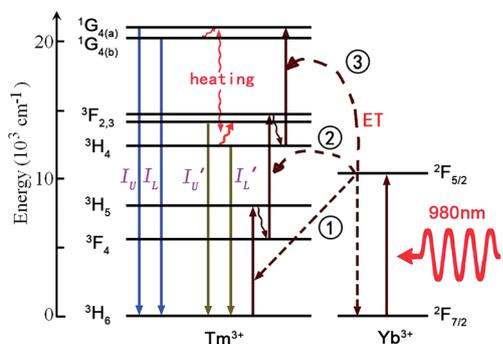
Fig. 6 The mechanism of optical thermal sensing through  $\text{Yb}^{3+}$ - $\text{Tm}^{3+}$  energy transfer under 980 nm infrared excitation.
