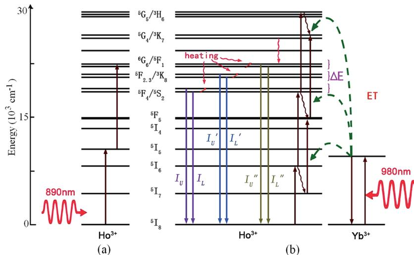
Fig. 9 The mechanism of optical thermal sensing through (a) up-conversion of the  $\text{Ho}^{3+}$  ion under 890 nm infrared excitation, and (b)  $\text{Yb}^{3+}$ – $\text{Ho}^{3+}$  energy transfer under 980 nm infrared excitation.
