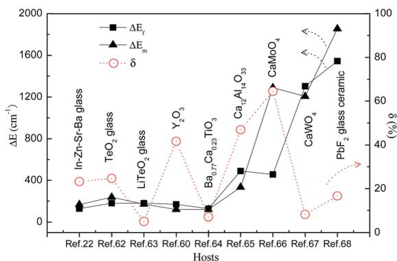
**Fig. 11** Host dependent  $\Delta E_T$  and  $\Delta E_m$  between the TCL of Ho<sup>3+</sup> ions, and the corresponding  $\delta$  values.
