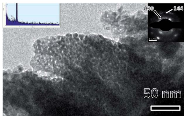
Fig. 2 Representative TEM micrographs of LaPO<sub>4</sub> nanoparticles synthesized using the citrate precursor route. Insets are EDS pattern (left top) and selected area electron diffraction (right top).
