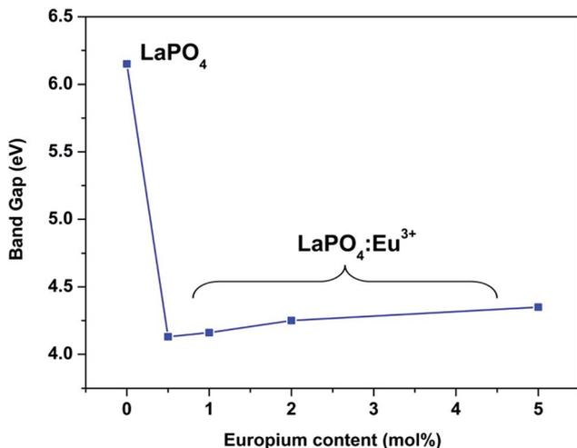
Fig. 16 The energy gap dependence of LaPO<sub>4</sub>:Eu nanoparticles on the Eu doping level.
