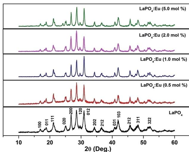
Fig. 1 XRD pattern of undoped and europium-doped LaPO<sub>4</sub> samples annealed at 800 °C.
