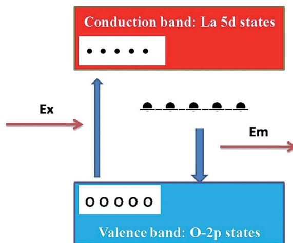
Fig. 5 Schematic model of probable mechanisms responsible for observed emission in  $\text{LaPO}_4$ . In the schematic model, the upper (red) and the lower (light blue) bands are La 5d conduction bands and O 2p valence bands, respectively. The black bar below the conduction band corresponds to the defect level created by the oxygen deficiency. White and black circles correspond to excited holes and electrons, respectively.
