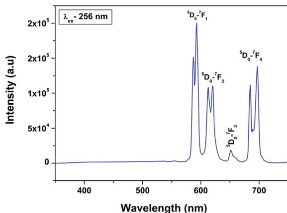
Fig. 6 Emission spectrum of LaPO<sub>4</sub>:Eu<sup>3+</sup> (0.5 mol%) at an excitation wavelength of 256 nm.
