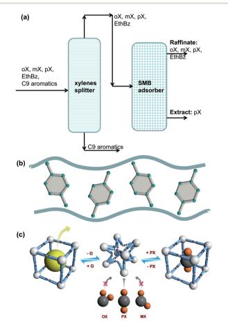
Fig. 27 (a) Schematic showing the separations of the oX/mX/pX/EthBz mixtures in a Simulated Moving Bed (SMB) unit. (b) Stacking of p-xylene within 10 Å channels of MAF-X8.<sup>84</sup> (c) Schematic representation of the framework flexibility of DynaMOF-100 with selective accommodation of p-xylene from xylenes mixture.<sup>4</sup>
