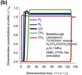
Fig. 15 Breakthrough characteristics of 5-component 73/16/3/4/4  $\rm H_2/CO_2/CO/CH_4/N_2$  mixture in adsorber packed with (a) Cu-TDPAT, and (b) UTSA-16a and maintained at isothermal conditions at 298 K and total pressure of 0.7 MPa.
