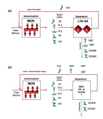
Fig. 23 (a) Currently employed processing scheme for nC6 isomerization and subsequent separation step using LTA-4A. (b) Improved processing scheme for the nC6 isomerization process.
