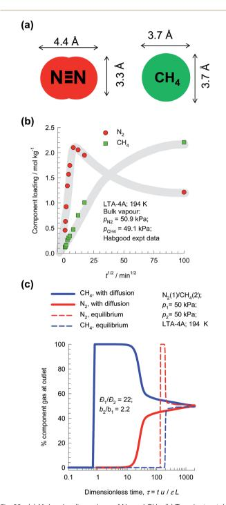
Fig. 22 (a) Molecular dimensions of  $N_2$  and  $CH_4$ . (b) Transient uptake of  $N_2/CH_4$  mixture in LTA-4A.<sup>76</sup> (c) PSA process for separation of 50/50  $N_2/CH_4$  mixture in a fixed bed adsorber packed with LTA-4A operating at a total pressure of 100 kPa and 194 K.
