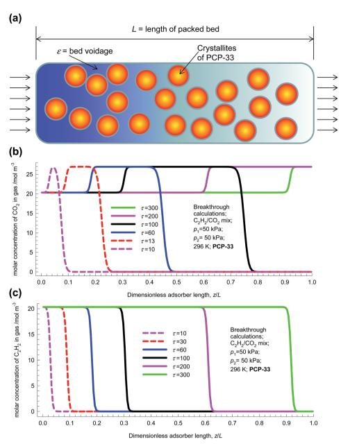
Fig. 4 (a) Schematic of fixed bed adsorber for C<sub>2</sub>H<sub>2</sub>/CO<sub>2</sub> mixture separations. (b and c) Transient development of concentrations of (b) CO<sub>2</sub>, and (c) C<sub>2</sub>H<sub>2</sub> along the length of the fixed bed adsorber.
