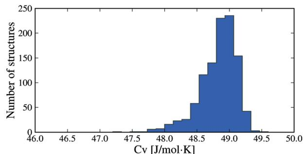
Fig. 6 Distribution of heat capacities calculated at 300 K for all 1061 crystal structures. Only intermolecular vibrational mode contributions are included.
