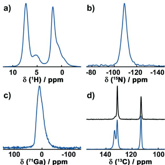
Fig. 3 Solid-state NMR spectra of Ga-CFA-6. a) DUMBO experiment of  $^1\text{H}$ ; b)  $^1\text{H}$ - $^{15}\text{N}$  cross polarisation experiment; c) Hahn echo spectrum of  $^{71}\text{Ga}$ ; d)  $^1\text{H}$ - $^{13}\text{C}$  cross polarisation experiment of the original sample (blue) and a sample dried under vacuum at  $250\text{ }^\circ\text{C}$  for 4 hours (black).
