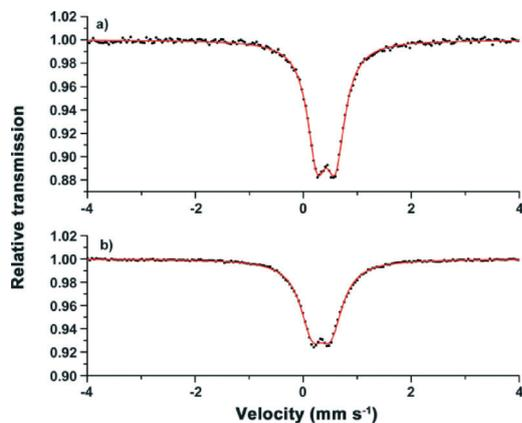
Fig. 8 Mössbauer spectra of Fe-CFA-6 recorded at 80 K (a) and 295 K (b). The symmetric shape of the doublet represents either exclusively  $\text{Fe}^{\text{II}}$  (LS) or  $\text{Fe}^{\text{III}}$  (HS) centres.
