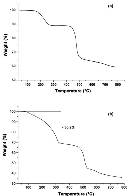
Fig. 4 Temperature profiles of Ga-CFA-6 (a) and Fe-CFA-6 (b). Ga-CFA-6 shows a weight loss between  $100$  and  $250\text{ }^\circ\text{C}$  resulting in a horizontal plateau. Decomposition starts at  $420\text{ }^\circ\text{C}$ . The weight loss of Fe-CFA-6 equals 30.2% between  $100$  and  $300\text{ }^\circ\text{C}$  (29.8% for one DMAc molecule per formula unit).
