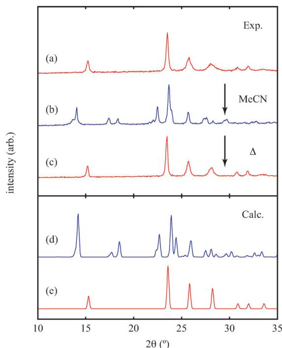
**Fig. 7** (Top) Powder X-ray diffraction patterns of (a) as-prepared Cu(tcm), (b) the same sample after exposure to MeCN, and (c) after subsequent heating at 200 °C for 3 h. (Bottom) Calculated X-ray diffraction patterns of (d)  $[\text{Cu}(\text{MeCN})(\text{tcm})]$  and (e) Cu(tcm).
