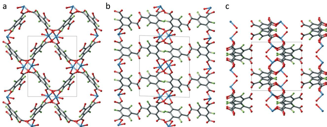
Fig. 4 Extended unit cell of UHM-33 along the *a*-axis (a), the *b*-axis (b) and the *c*-axis (c); grey: carbon, red: oxygen, blue: copper, green: fluorine, hydrogen atoms and solvent molecules are omitted for clarity.
