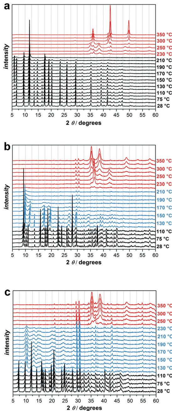
Fig. 5 Variable temperature powder XRD pattern of UMH-31 (a), UHM-32 (b) and UHM-33 (c). For each experiment 23 diffractograms were measured, the first three ones at 28, 50 and 75 °C, followed by temperature steps of 10 °C from 100 up to 250 °C and steps of 25 °C up to 350 °C. Black represents the original MOF phase, blue the new MOF phases and red the decomposition products. The two reflections at  $2\theta = 29.4$  and  $2\theta = 30.5$  are probably caused by the sample holder.
