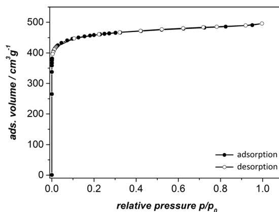
Fig. 7 Nitrogen physisorption isotherms of activated UHM-31 measured at 77 K.
