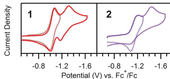
**Fig. 2** Cyclic voltammograms of 0.20 mM **1** and **2** without acid at 100 mV s<sup>-1</sup> and with 0.1 M [Bu<sub>4</sub>N][PF<sub>6</sub>]. The  $Ni^{II}/Ni^I$  reduction of **1** is reversible (dotted trace) and the  $Ni^I/Ni^0$  reduction is quasi reversible. The  $Ni^{II}/Ni^I$  reduction of **2** is reversible (dotted trace); however the  $Ni^I/Ni^0$  reduction is irreversible.
