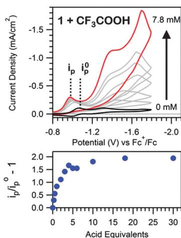
**Fig. 1** Top: voltammograms of 0.39 mM **1** with additions of 0 to 20 eq. (7.8 mM) of CF<sub>3</sub>COOH at 100 mV s<sup>-1</sup> in a 100 mM [Bu<sub>4</sub>N][PF<sub>6</sub>] CH<sub>3</sub>CN solution. Bottom: the peak current of the prewave relative to the one-electron reduction of the catalyst in the absence of acid ( $i_p$  = peak current,  $i_p^0$  = peak current of  $Ni^{II}/Ni^I$  reduction in absence of acid).
