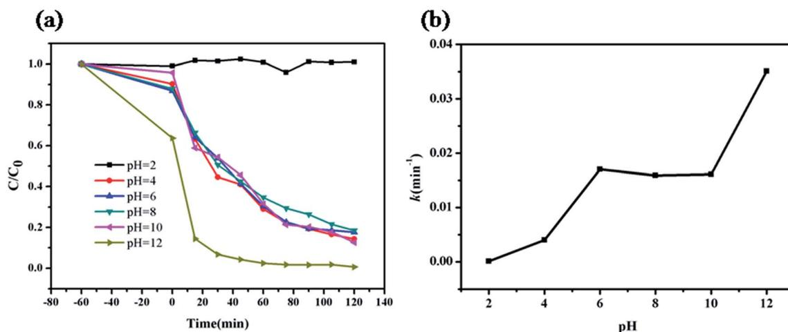
Fig. 5 (a) Effect of initial pH on the degradation of MB. Experimental conditions: ZIF-8,  $0.5 \text{ g L}^{-1}$ ; MB,  $10 \text{ mg L}^{-1}$  and UV irradiation. (b) The corresponding pseudo-first-order rate constants for system with  $\text{pH} = 2.0$ – $12.0$ .
