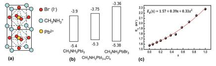
Fig. 14 Structure and energy levels for perovskites used in solar cells. (a) Unit cell for  $CH_3NH_3PbI_3$  and  $CH_3NH_3PbBr_3$  perovskites. (b) Energy levels for  $CH_3NH_3PbI_3$ ,  $CH_3NH_3PbI_3$ ,  $CH_3NH_3PbI_3$ ,  $CH_3NH_3PbI_3$ . The energy levels for the latter were taken from ref. 209, 210 and 211 respectively. (c) Variation of  $E_g$  with Br composition for  $CH_3NH_3PbI_3$ . (c) reproduced with permission from ref. 208.
