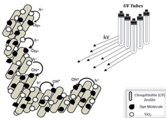
Fig. 8 Synergistic effect of TiO<sub>2</sub> and clinoptilolite catalyst on dye degradation by producing OH free radicals.<sup>318</sup>
