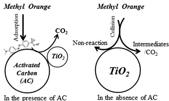
Fig. 9 Synergistic mechanism between AC–TiO<sub>2</sub> composites. The arrow labelling un-reacted emphasizes that in the absence of Absorbent the reactants may remain un-reacted into the solution resulting in low photoactivity of methyl orange.<sup>236</sup>
